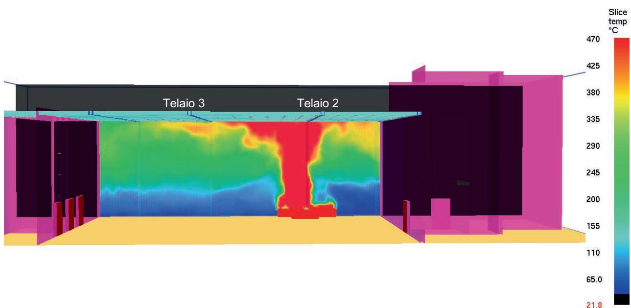
**SLICE DI TEMPERATURA A  $Y = 1,20 \text{ m}$  IN CORRISPONDENZA DEL MATERIALE COMBUSTILE,  $T = 1000 \text{ s}$**
